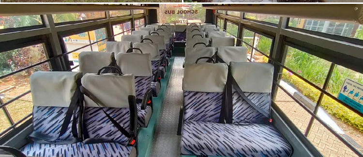
3 point seat belts installed in the big School bus
